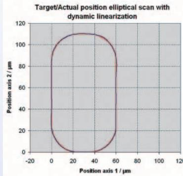
The same scan as before but with a DDL controller. The tracking error is reduced to a few nanometers, target and actual position cannot be distinguished in the graph
