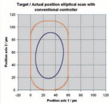
Elliptical scan (for laser micro bore applications) with an XY piezo scanning stage and conventional PID controller. The outer curve shows the desired position, the inner curve shows the actual motion
