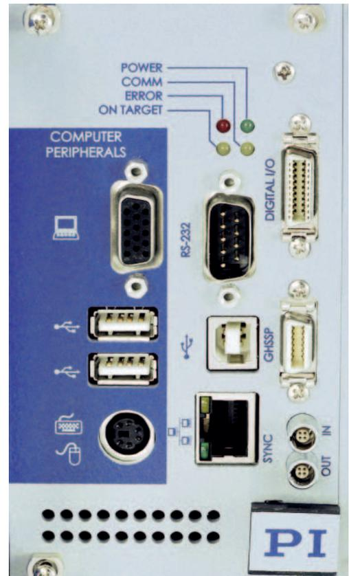
The standard interfaces for digital nanopositioning controllers are RS-232, USB and TCP/IP. Additionally, PI offers digital I/O lines, options for analog interfaces and real-time PIO
