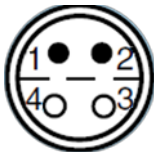
Figure 14: Sensor connection: LEMO connector FFA.05.304.CLAC32Y, contact side
