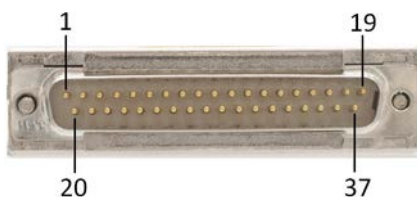
Figure 15: Voltage and sensor connection, sub-D 37 (m)
